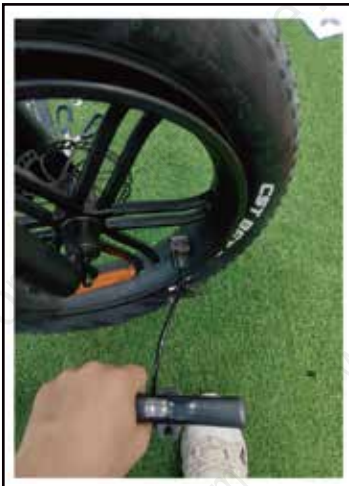
17. Fill the tires with air
